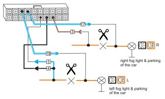
2. Wiring diagram for realized the functions on a single filament light bulbs parking 6 Volt and stop 12 Volt
