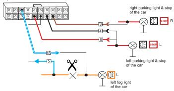
Wiring diagram for realized the functions on a single filament light bulbs fog 12 Volt with add a resistive load MH3-REZ in BMW, MERCEDES, VW
