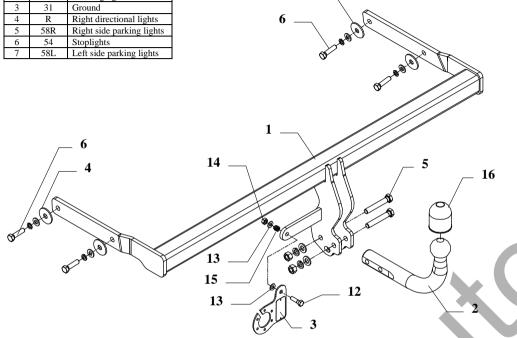
This towbar is designed to assembly in following car: RENAULT MEGANE II, 4 doors, produced since 09.2003 till 10.2012, catalogue no. G43 and is prepared to tow trailers max total weight 1300 kg and max vertical load 75 kg.
