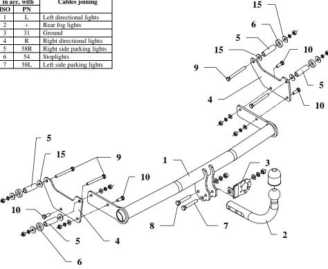
This towing hitch is designed to assembly in following cars: RENAULT MODUS/GRAND, 5 doors, VAN, produced since 02.2008, catalogue no. G59 and is prepared to tow trailers max total weight 1200 kg and max vertical mass 75 kg.
