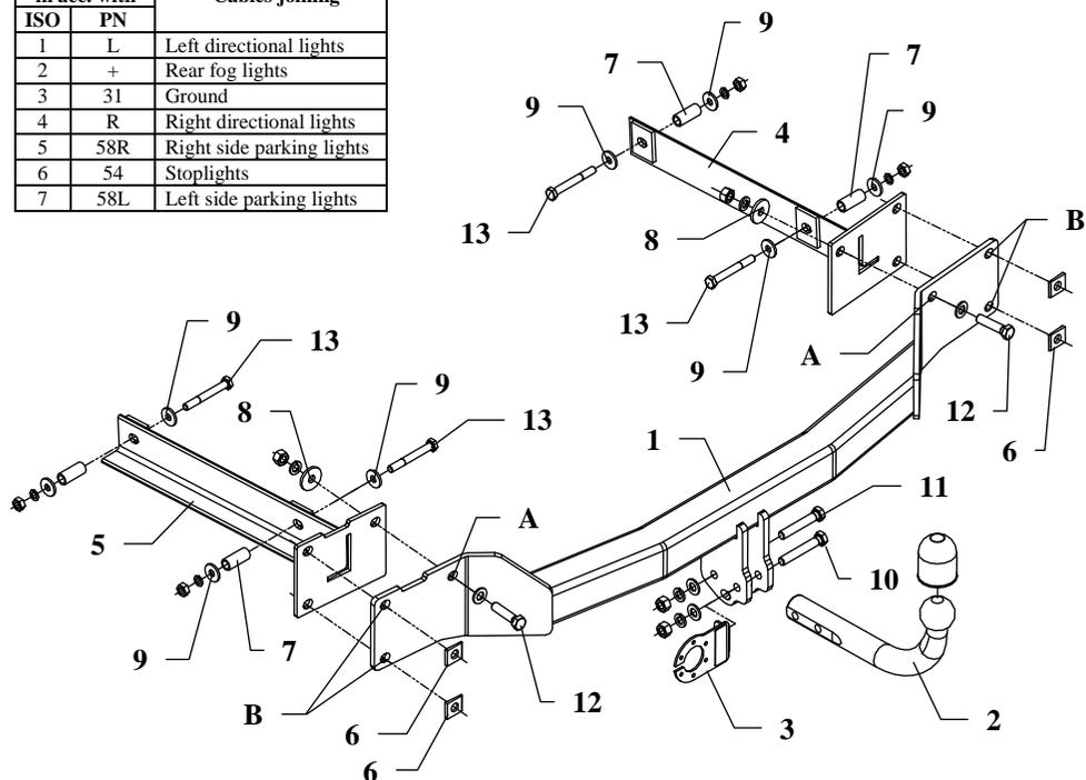
This towing hitch is designed to assembly in following cars: **MERCEDES S-CLASS, (W220), except AMG**, produced since 1999 till 2005, catalogue no. **D36** and is prepared to tow trailers max total weight **2100 kg** and max vertical load **85 kg**.
