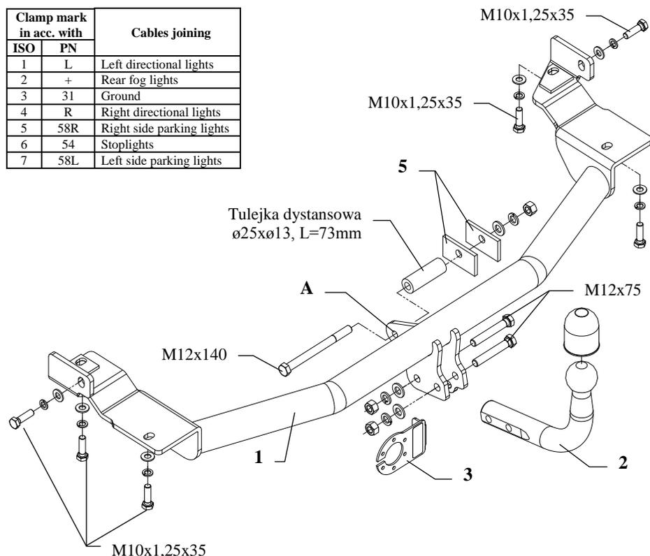
This towbar is designed to assembly in following car: **MITSUBISHI SPACEWAGON, VAN (N5, N8, N9)**, produced since 11.1998 till 04.2004, catalogue no. **Z27** and is prepared to tow trailers max total weight **1600 kg** and max vertical load **80 kg**.
