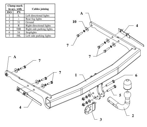
This towing hitch is designed to assembly in following cars: **FORD MONDEO, 5 door (Mk4),** produced since 05.2007 till 09.2014, catalogue no. **C54** and is prepared to tow trailers max total weight **2120 kg** and max vertical mass **80 kg**.
