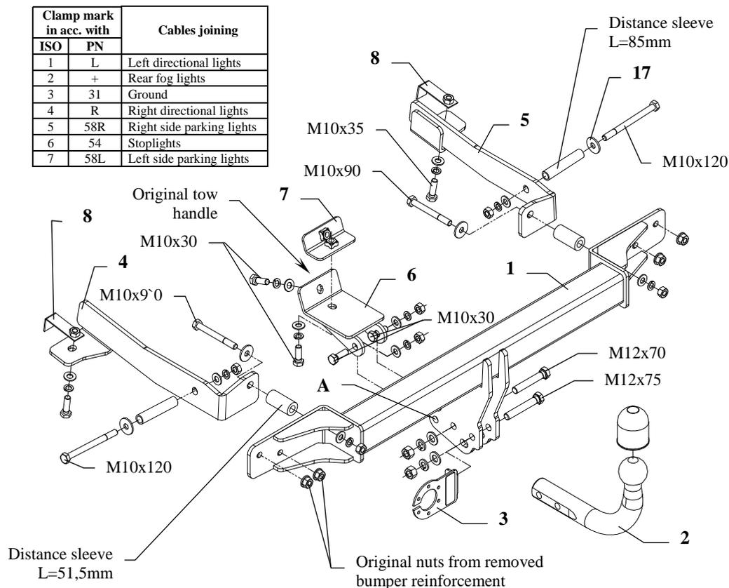
This towing hitch is designed to assembly in following cars: **HONDA ACCORD TOURER, Estate (CM1, CM2, CN2), except Type S and except 2,4L engine**, produced since 05.2003 till 07.2008, catalogue no. **Y28** and is prepared to tow trailers max total weight **1500 kg** and max vertical load **75 kg**.
