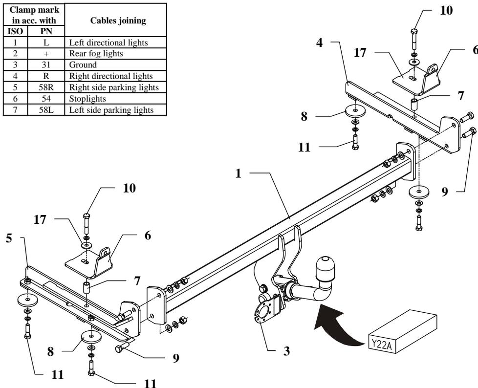
This towing hitch is designed to assembly in following car: **HONDA ACCORD 4/5 doors (CD7, CD8, CD9)**, produced since 03.1993 till 10.1998, catalogue no. **Y22A** and is prepared to tow trailers max total weight **1400 kg** and max vertical load **70 kg**.
