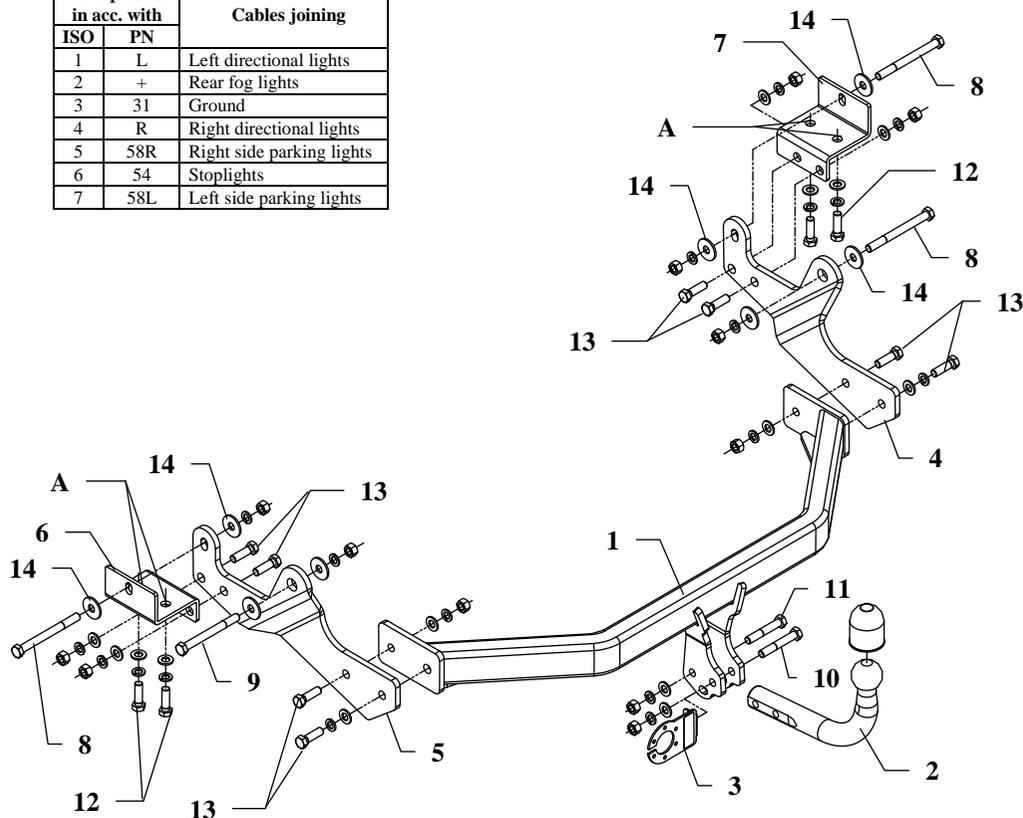
This towing hitch is designed to assembly in following car: **HYUNDAI H1/H300, H1 STAREX, VAN and MINIBUS** produced since 02.2008, catalogue number **J58** and is prepared to tow trailers max total weight **2300 kg** and max vertical mass **100 kg**.
