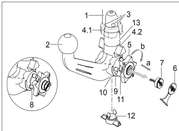
**Posición enclavada, lista para circular**
