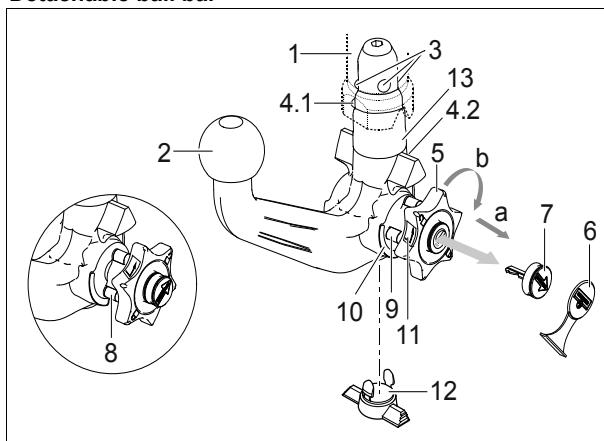
**Locked position, operating condition**
