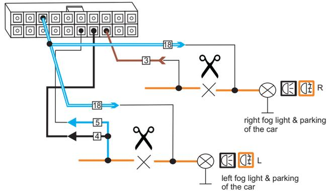
2. Wiring diagram for realized the functions on a single filament light bulbs parking 6 Volt and stop 12 Volt
