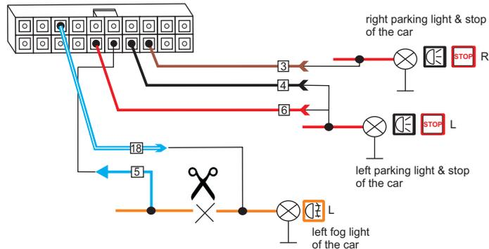
3. Wiring diagram for realized the functions on a single filament light bulbs fog 12 Volt with add a resistive load MH3-REZ in BMW, MERCEDES, VW
