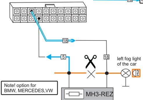
Note! 18 pin output to connect in the car for fog lamp left PWM control
